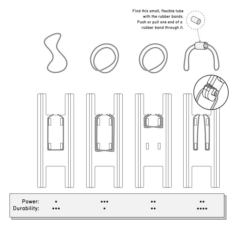
There are several different ways to attach a rubber band to your catapult. Higher power means longer range. Lower durability means rubber bands will snap more often.
